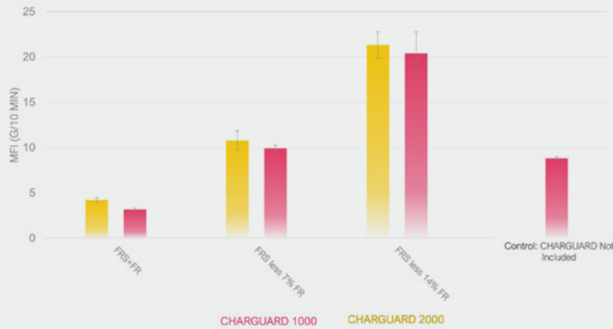
FIGURE 3: Melt flow index via ASTM 1238 (210C / 2.16kg.)
