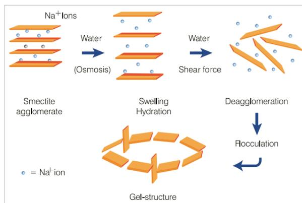
BENTONE® rheological additives improve suspension properties and are easy to handle. They are also suitable for applications requiring fast water release and exceptional sag resistance. In construction applications, they give easier workability for tile adhesives, grouts, skim coats and mastics. Examples of very different types of modified clays are listed below.
