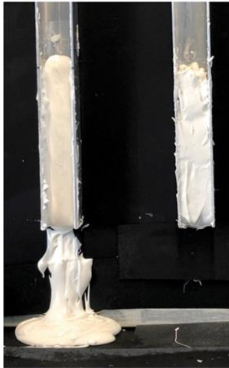
Improved Sag Properties with the Diamide-based Thixotrope (right) compared to Fumed Silica at Equal Loading of 1.0%.
