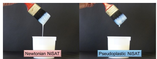
Figure 21: NiSAT effect on dripping
