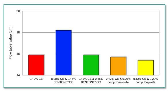
For all clay additives equal spread rates of around 16 cm are observed when formulated with an equal amount of 0.12% of the original cellulose ether content. The sample with lower cellulose ether content demonstrates significantly lower consistency and is therefore not of practical use.
