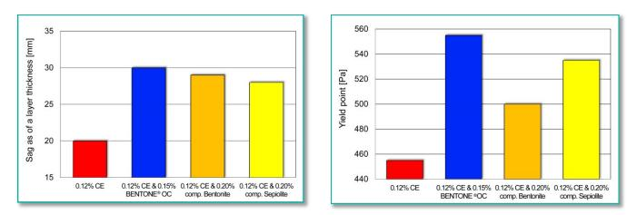
The highest sag stability and yield points are obtained with BENTONE<sup>®</sup> OC, both compared to competitive clays as well as to the formulation with cellulose ether only. This means thicker stable layers can be applied on the vertical surface without sagging.
