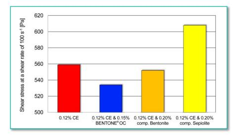
The formulation with BENTONE<sup>®</sup> OC requires the lowest amount of energy to initiate flow at a shear rate of 100 s<sup>-1</sup>. The competitive Bentonite grade shows also better results in comparison to the formulation with cellulose ether only. The competitive Sepiolite, shows even poorer results than the formulation with cellulose ether only.
