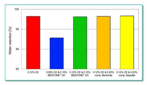
Water retention was tested using the filter plate method, in accordance with DIN 18555, Part 7.
