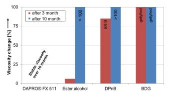
Data displayed are showing that only with DAPRO FX 511 stable viscosities could be acieved in a silicate based paint. The use of all other tested coalescents resulted in a tremendous viscosity rise.
