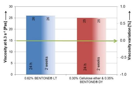
BENTONE<sup>®</sup> LT is a grade which could be as a stand alone alternative to a combination out of cellulose ether and Xanthan gum. BENTONE<sup>®</sup> DY is typically formulate as a partial replacement for cellulose ether.
