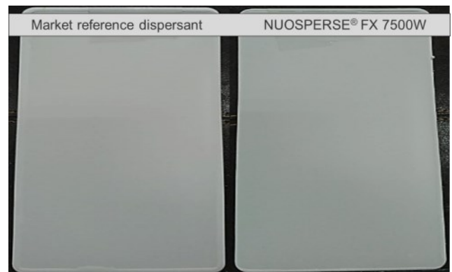
Figure 12: Corrosion prevention at high humidity
