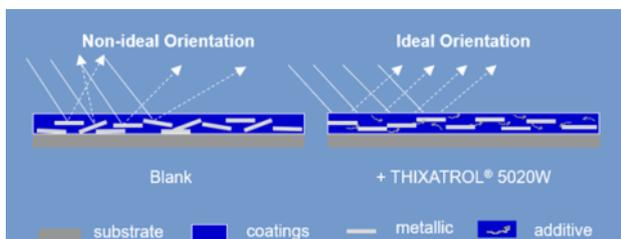
Figure 1: Metallic orientation mechanism
