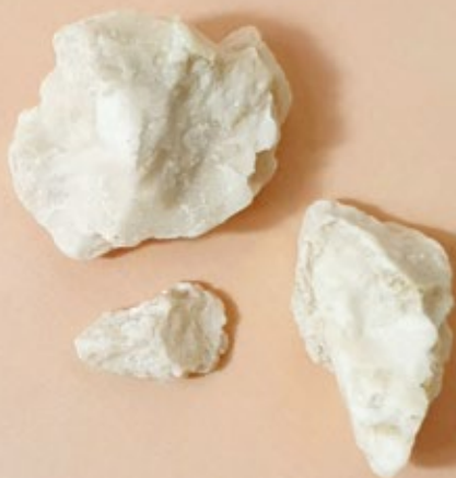
Hectorite is a natural white clay mineral, with a layered 'house of cards' molecular structure.
